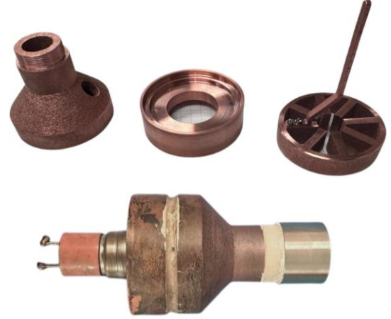
Figure 4: Post-Processed 3D-Printed Magnetron Parts and Fully Assembled Magnetron
