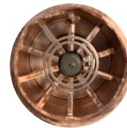
Figure 1: Cross-Section of the reference 2M214 magnetron
